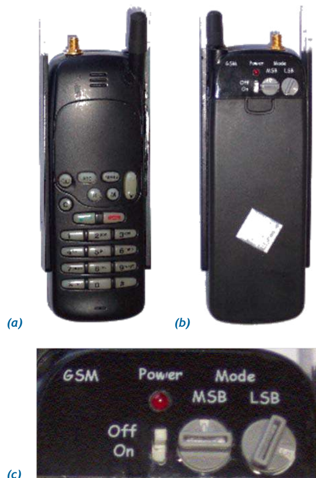
FIGURE A1 (a) front, (b) back and (c) control switches of the GSM phone exposure system
